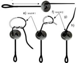
h) Minimum tail length on stretched loop: Please keep the loop-tail like it is and just tuck it away. Be aware that if you like to cut it off or shorten the tail, please use a hotknife to avoid freying and make sure that the piece it is not too short which could loosen the knot.
