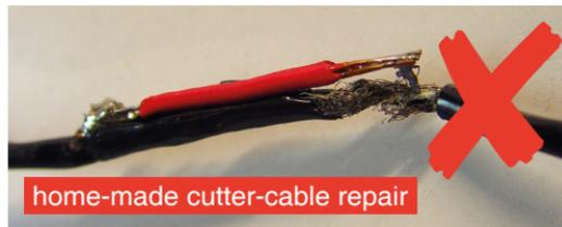
With a damage like this, the CYPRES will most likely still function like usual, but with the broken metallic, electrostatic shielding, it could result in a failing control unit. display. Please return for repair.
