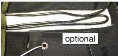
the container bottom. This is optionally and it must be assured that the cable will stay inside this channel at all times and does not interfere with any function of the reserve / container system and deployment.
