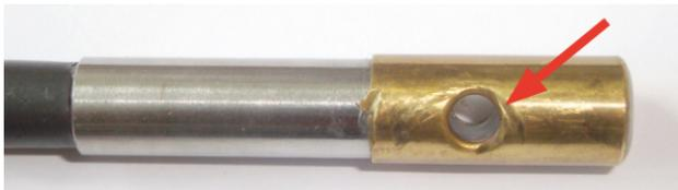
CYPRES cutter in unacceptable condition. The only option here is to send it to Airtec GmbH & Co. KG Safety Systems or SSK for repair. \* There the brass sleeve will be replaced free of charge and returned back to the owner in perfect condition.
