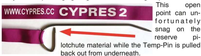
To avoid damages on reserve pilotchutes, you can cover up this part using a 4 inch piece of webbing and attach it like shown.
